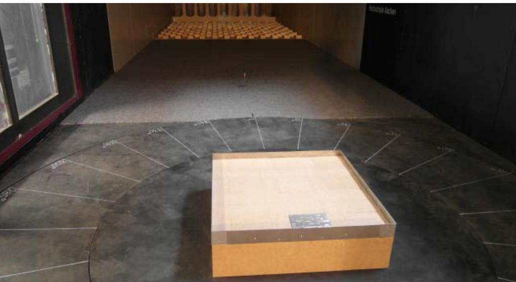
Wind tunnel model of a flat-roofed building with parapet and an array of a solar ballasted roof mount system on a scale of 1:100 in the large I.F.I. boundary layer wind tunnel.
